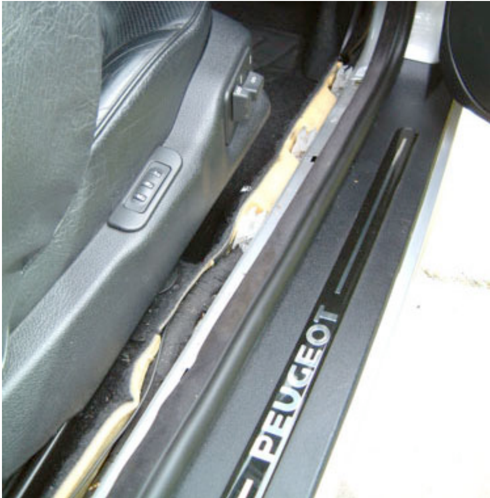
Routing the cable with the trim removed
